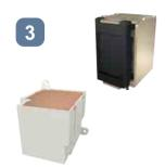
This is the device that automatically trips the breaker when the circuit voltage drops below the nominal voltage, and comprises a UVT coil and UVT controller. There are 3 kinds of tripping time, INST, 0.5s and 3.0s.
